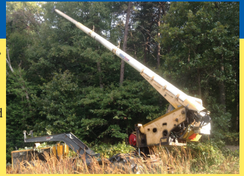
This mechanical tree trimmer will be working in rural areas to keep NOVEC's right-of-way areas clear for easy access during repair and maintenance work.
